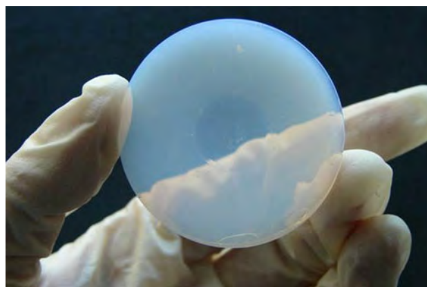
Fig. 11 Example of silica aerogel monolith (sample synthesized by a two-step catalytic process from TEOS and dried with supercritical \text{CO}_2 , presenting a density of 0.13 \text{g cm}^{-3} and an effective thermal conductivity of 0.015 \text{W m}^{-1} \text{ K}^{-1} as respectively measured by mercury pycnometry and with the hot-wire method at room temperature)
